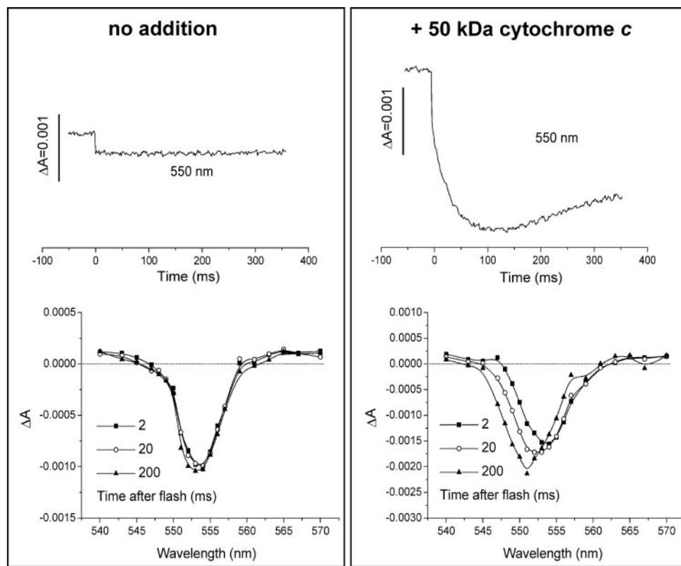
**FIGURE 4. Flash-induced absorbance changes of cytochrome *c* in the membranes in the presence or absence of the extra 2  $\mu$ M 50-kDa cytochrome *c*.** Membranes were suspended to  $OD_{854} = 1.0$  in a buffer containing 20 mM MOPS-NaOH (pH7.0) and 100 mM KCl. The membranes were treated with 0.04% Triton X-100 to remove native membrane-bound 50 kDa cytochrome *c*.
